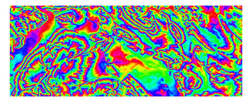
complex multiplication of the two images; i.e. the corresponding amplitudes have to be averaged and the corresponding phases have to be differenced at each point in the image
