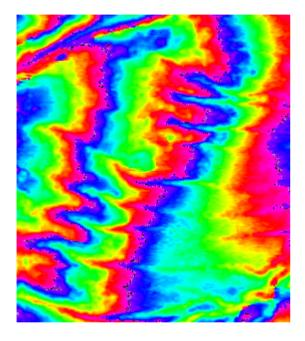
represents the whole range of the phase in an interferogram from 0 to 2π in a full color cycle
