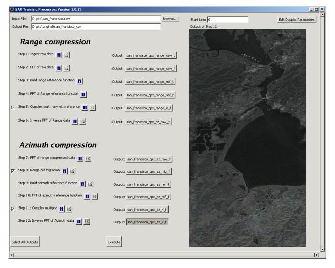
A closer examination of our initial result shows that the image is not crisp and well focused. As it turns out the level zero processor had severe difficulty determining the Doppler centroid based on the contents of just this particular frame.
