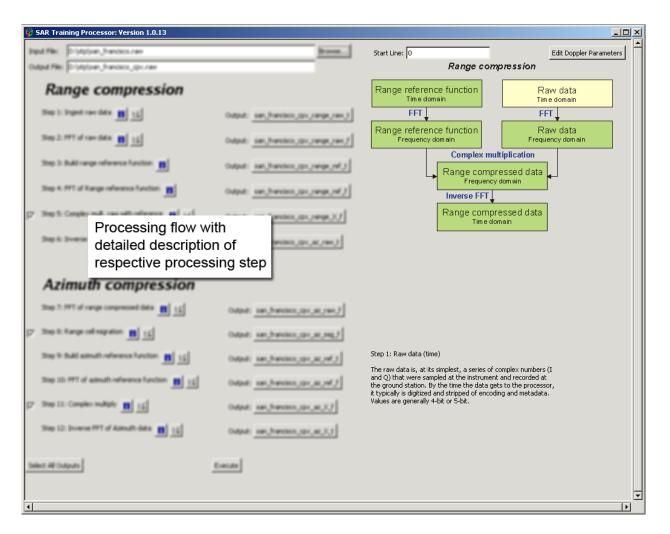
Each processing step is explained in detail with a diagram showing the place of the processing step within the general SAR processing flow. This way the user has the context how the particular processing step fits into the overall processing scheme. The information buttons next to the processing steps are used to switch between the descriptions of the individual steps.
