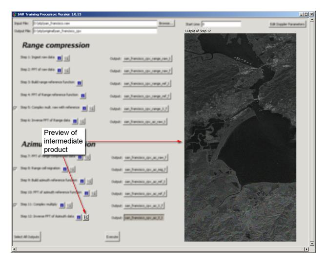
The output of each processing step can be visualized using the preview button located next to the information button. For closer examination of the intermediate results the user can view the JPEG images in the common graphics or image processing packages.
