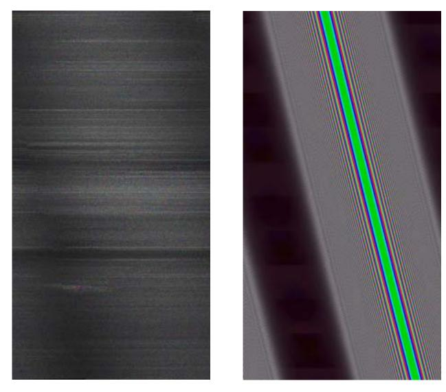
The use of the range cell migration can only be demonstrated in frequency domain (on the left). Moving all responses of a target from the trajectory into a straight line in time domain leads to a shift in frequency domain. The angle of this frequency shift, caused by the Doppler, follows the one in the azimuth reference function (on the right). All individual point targets are now lined up in straight lines.
