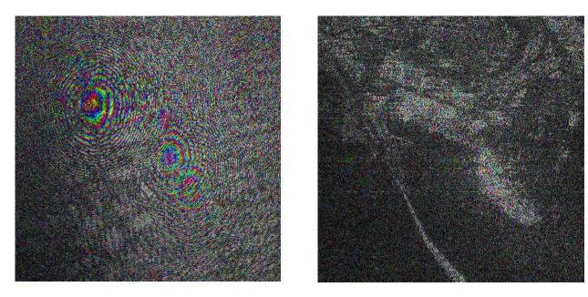
The bright point targets that can be identified in the processed SAR image (on the right) show up as bulls eyes in the raw image (on the left). The amplitude part of the signal does not offer much of an indication for point targets.
