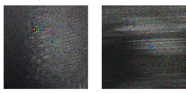
The bright point targets in the range compressed image (on the right) now can be identified a lot easier in the amplitude part of the signal (compared to the raw image on the left) as they show up as elongated bright streaks. The water body is more clearly delineated from the land mass.
