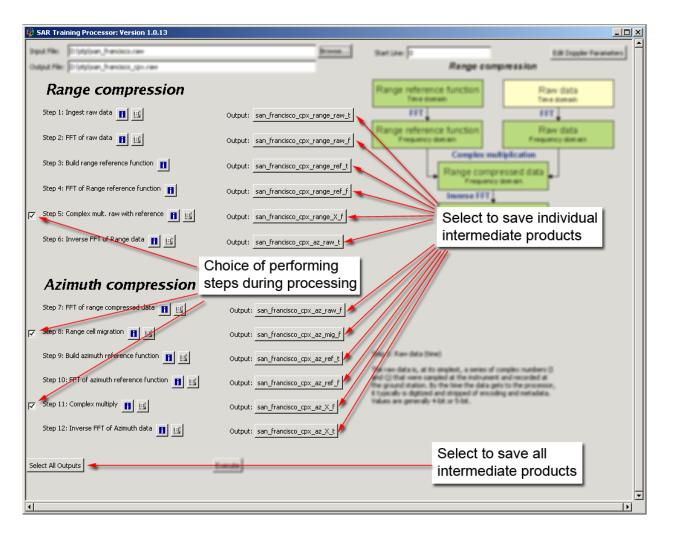
The range Doppler processing consists of two compressions in range and azimuth direction, i.e. two complex multiplications with the respective reference function, and a correction for range cell migration. For a well focused SAR image all these three processing steps need to be carried out. However, the user can study the influence of leaving any of these steps out of the processing flow by changing the status of the check box next to the processing steps.
