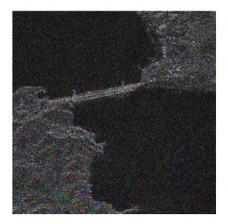
Comparing the two results (processing without range cell migration on the left, processing with original Doppler values on the right) shows that processing without range cell migration leads to a severe defocusing of the image, even more than the processing with a wrongly estimated Doppler centroid.
