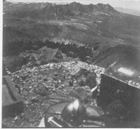
Fig. 3. Millikan-Neher type cosmic ray electroscope, in 10 cm lead shield, on top of El Misti, 19200 feet (about 5850 meters) in southern Peru.
